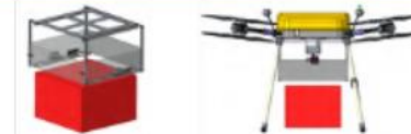
Step 2 : After parcel falling, the Torsion springs will close the door, door sensors sensed and servomotors lock the doors, ultrasound sensor double confirm parcel fallen, then drone takes off and flies back.
