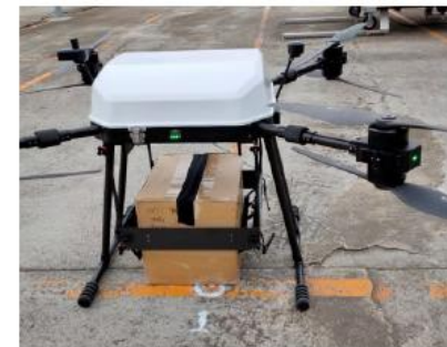
Step 1 : After drone landing, the servomotors release the unloading doors, and the parcel falling from the catcher.
