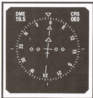
FIGURE 123.—Aircraft Course and DME Indicator.
