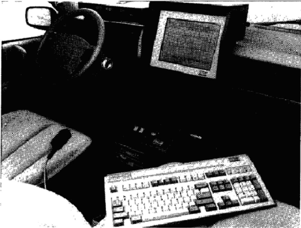
圖 5-7 The vacuum florescent display unit and keyboard for the Runway Friction Tester van
