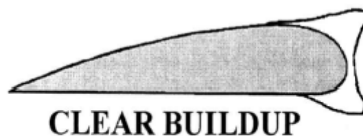
Figure 5. Clear ice buildup with horns.
